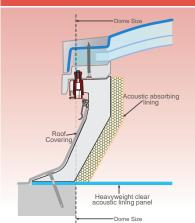
The Acoustic Pack is effective in reducing rain noise penetration (LiA) by over 15dB to 47dB.
